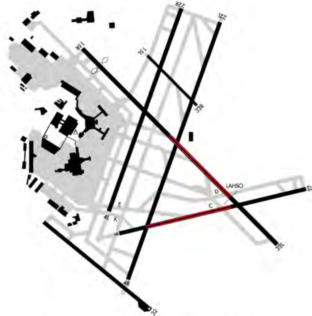
Figure 3. Runway Intersection Lights (RILs) Locations on 15R and 9
