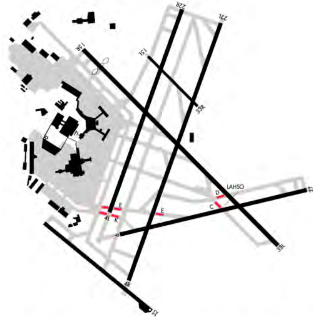
Figure 1. Runway Entrance Lights (RELs) Locations on 4L/22R, 4R/22L, 15R/33L, and 9/27
