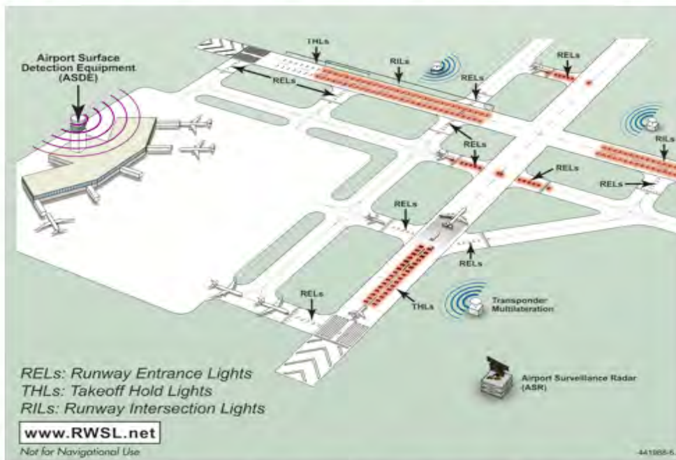
Figure 7. Conceptual diagram of the Runway Status Light System with surveillance sources driving RELs, THLs, and RILs shown illuminated in red
