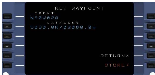
Figure 1. Example FMC Display: Full Waypoint Latitude and Longitude (13-characters) inserted into FMC
