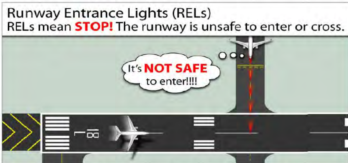
Above: the lights indicate the presence of an airplane on an active runway.
